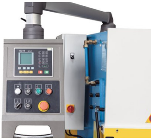
NC control for quick positioning of the back gauge
