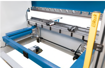
Option: Back gauge with controlled R axis
