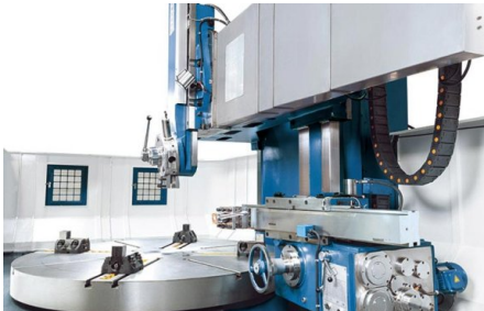
Vertical support includes a 5-station tool holder, side support with independent feed for inside and outside turning
