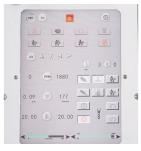
The high-resolution touchscreen features a scratch-resistant surface. Matching rpm and feed speeds for each drill can be recalled from a database and automatically applied.
