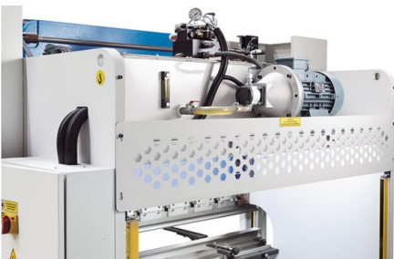
Hydraulic unit positioned on the top of the machine for extra bending space.
