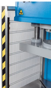
The workspace is protected by light curtains
